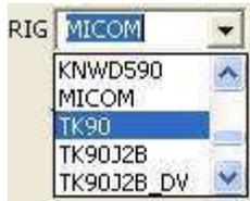
The CAT serial port parameters are automatically configured when the radio type is selected, the fast baud rate should always be used to minimize latency.
