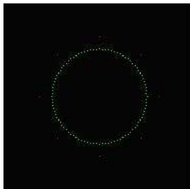
In a perfect world the GREEN pixels or when E mode is enabled the ORANGE pixels would be directly over the RED pixels in a tight cluster so much so the RED pixels would not be seen. The boundary pixels are almost never going to rotate or otherwise move until we reach the point in the equalizer when things fall apart so bad and so fast you lose DCD and even then you won't often see them change with the naked eye.
