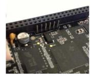
Just what if any use this port may be in the actual BBB-ALE implementation aside from debugging is to be determined. Its a direct connection to an FTDI and is always active however.
