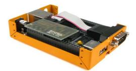
It can hold not only the CBB-TTL-232 board and its ribbon cable but should also hold the codec PCB with TXCO option that is of interest for data modem adhered to the serial board for use as pictured in the mockup image below.
