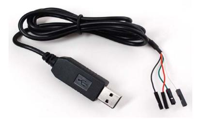
There are four wires with the Adafruit cable: Red power, Black ground, White RX into USB port, and Green TX out of the USB port. The power pin provides the 5V @ 500mA direct from the USB port and the RX/TX pins are 3.3v signal level vs. 5v TTL. Where the Red wire D.C. power connection from the USB port of the PC is not required as seen below.
