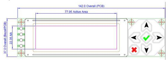
End users with the ability and cost savings incentive can make their own cut out panels and bezel, all the details are provided from the manufacturer in the form of drawings and templates. The 6 keys are Up, Down, Left, Right which are obvious, Enter being the green check mark in the center and Exit being the red X button. The Keypad on units with it integral is also used for Power On via the Enter key and Power Off via the X key as desired.
