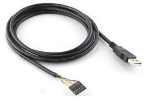
is required (<u>http://www.ftdichip.com/Support/Documents/DataSheets/Cables/DS\_TTL-232R\_CABLES.pdf</u>). Pin 1 on the cable is the black wire and connects to pin 1 on the debug header on the BBB. If there is a use for the debug port in BBB-ALE all the time with the PC then this cable would likely be the best route to take where it would be fished out the case.
