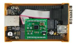
The pop out switch hole next to the ethernet port connector can be used to bring out a cable with ground, audio in/out and radio PTT lines retained with a nylon tie on either side of the case or perhaps a connector like PS/2 mouse or S-Video could be used.
